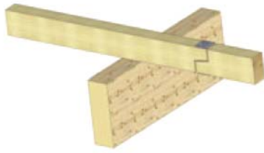
Pannes à joints Gerber (Cantilever)
